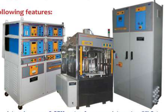
Internal pressure & CRM system for vacuum interrupters (VI) Set
