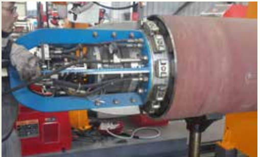
Pneumatic Pipeline Internal Line-Up Clamp
