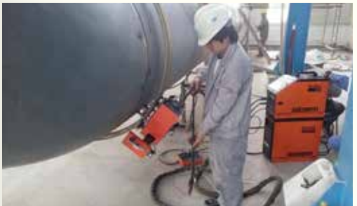
Piping All-position Automatic Welding Machine(Rail Type)
