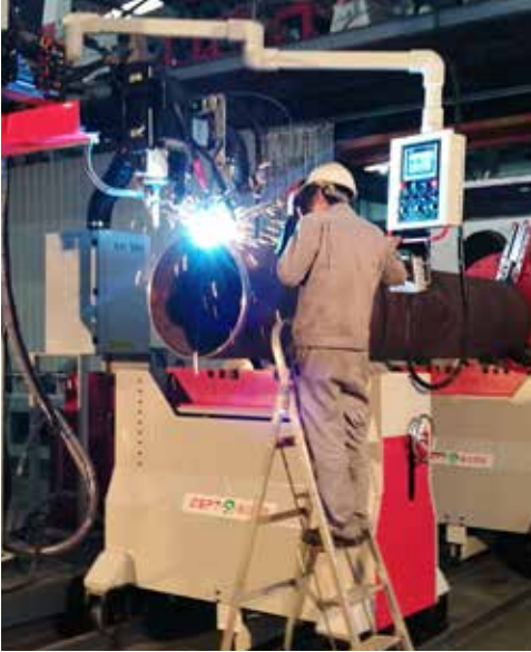
7、自动焊机焊接性能试验 Automatic Welding Machine Welding Performance Test
