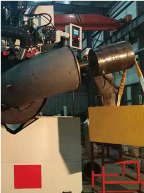
3、厚壁焊机旋转扭矩测试 Regular Welding Machine Rotating Torque Test
