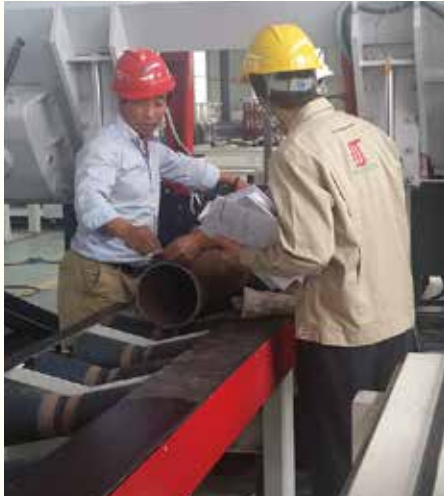
1、带锯床定长精度测试 Band Saw Machine Length Measurement Precision Test
