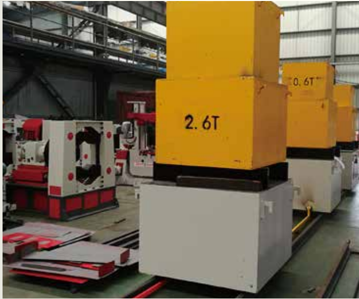
5、轨道小车运输能力测试 Rail& Trolley Conveying Capability Test
