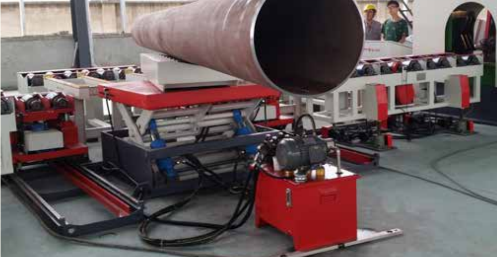
6、调头机构调头能力测试 U-Turning Mechanism Capability Test
