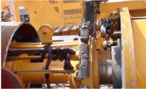
Pipeline Internal-Expanding End Beveling Machine
