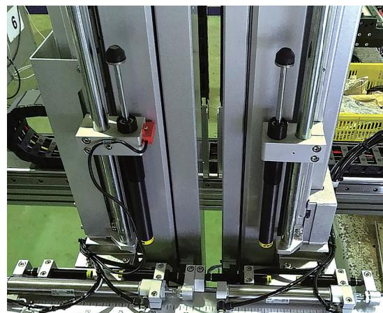
CEC SHOCK ABSORBERS USING IN ROBOT PICKER
