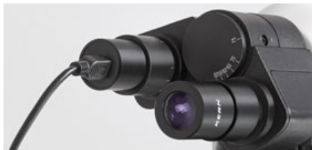
Eyepiece camera fixed into the tube
