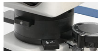
Bertrand lens, \lambda Slip, 360° rotatable analyser (removable)
