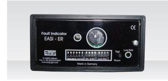
Combined short circuit and earth fault can be also provided. The indicator set consists of one reading instrument, four sensors (one sensor on the 3 core cable and three for the individual 1 core cables) and four fibre optic/standard copper cables. Earth fault and short circuit can be indicated
