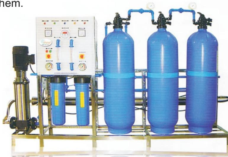
Operation Of Water Softening Plant In the long run of usage when these softeners are covered with these hard ions, the water softeners will start to lose its ability to do its work however through a process called regeneration, it will be about to continue its softening process from salt (Brine Solution).
