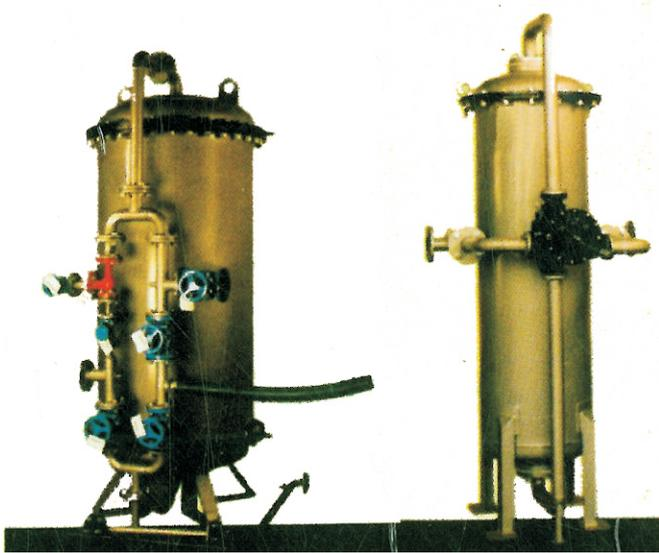
The raw water passes through a bed filled with small polystyrene beads known as ion exchange resins where sodium ions are exchanged for hardness forming ions. Once the beads are saturated with calcium and magnesium, the unit enters a regenerating cycle.
