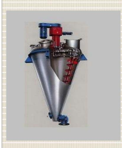
Cone screw mixer is widely used in chemical, food, cosmetic and pharmaceutical industries. The floor space required for this type of mixer is very less and they can be started on full load. The material of various densities, sizes and particle shapes are also mixed homogeneously without any degradation. The screw rotates about its own axis and revolves along the walls of the cone. Due to the conical shape the unloading of the material is helped by gravity and is complete without any hold-up.
