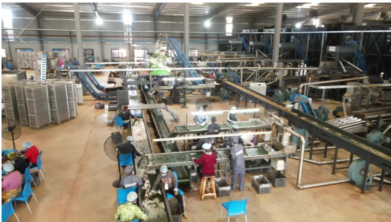
RCN Shelling and Separating Section
