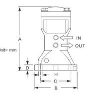
FREQUENCY (V.P.M.) FORCE (N) AIR WEIGHT Model No. CONSUMPTION (g) 2kg/cm 6kg/cm<sup>2</sup> 2kg/cm<sup>2</sup> 4kg/cm<sup>2</sup> 6kg/cm  $(\ell / \min)$ 4kg/cm BVP10000-0130 1900 2800 3500 3600 5400 6200 250 1.0 kg BVP10000-0140 2.1 kg 1700 2400 3000 6450 8750 9400 270 BVP10000-0160 1200 1800 1900 6900 12850 13850 300 4.8 kg
