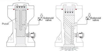
(1) Compressed air via top airbreathing tube pushes piston moving downward. Air in the bottom will be exhausted via outlet hole.
