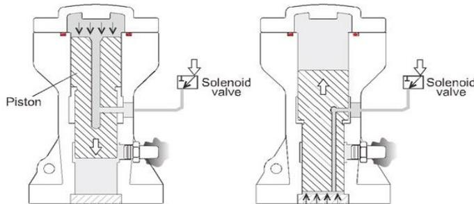
(1) Air is compressed into the body to push piston move downward. Air in the bottom side will be exhausted by the outlet hole.
