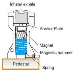
(2) The hammer instantly drops down when air pressure overcomes the strength of Magnet to cause a downward impact.
