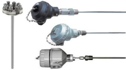
Industrial thermocouple assemblies are designed to be used in the most severe and demanding environments. The choice of a specific style is to a large degree determined by the temperature working range, ambient atmospheric or media conditions, as well as the size and shape required for the application. Control requirements such as accuracy and speed of response may also be taken into considerations.
