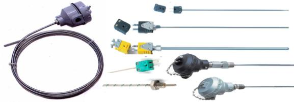
Thermocouples with magnesium oxide insulation are recommended where the thermocouple is immersed in liquids, high moisture, corrosive gases, or high pressure. The thermocouple can be formed to reach otherwise inaccessible areas. The magnesium oxide has a high dielectric strength, responds quickly to temperature changes, and is very durable.
