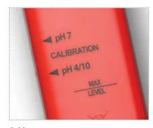
Guides The max level guide lets you know how deep to submerse the probe.
