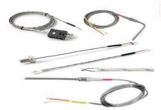
Bayonet thermocouples have a compressible spring and locking cap for quick insertion and detachment. Other probes connections like washer, button, plate, ribbons, ball, nozzles, bolts etc are beings used to manufacture flexible thermocouple to suit various critical temperature measuring applications.
