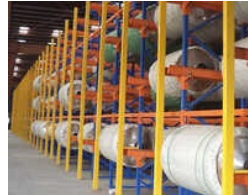
Gravity Flow Racking
