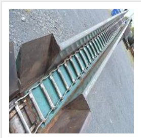
Boiler Drag Chain Feeder Assembly
