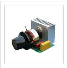
HVAC Speed Controller
