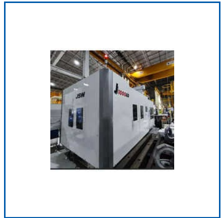
JSW J1000AD-3100H INJECTION MOLDING MACHINE
