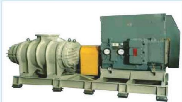
Process Air Blower-41000 cmh, Pressure of 0.88 Bar driven by 1300 kw motor.
