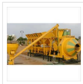
Automatic Batching Mixer Plant
