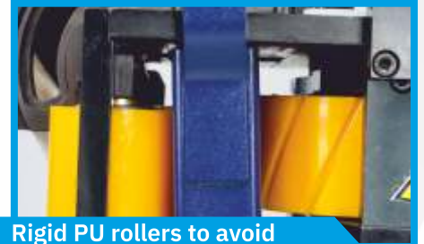
Rigid PU rollers to avoid Impression mark on Job
