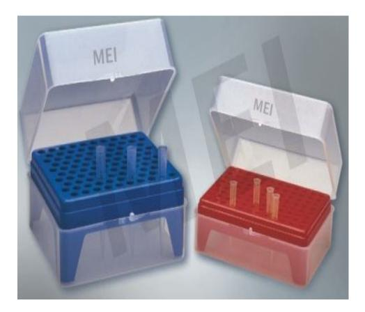
These unique boxes are molded in Polypropylene and are therefore autoclavable. The Box itself is clear providing on excellent view on the tips inside while a table like structure is provided inside to hold the tips. The tip holding spaces are uniformly placed to facilitate the use of multi channel pipettes. The cover is joined to the base through ball catcher hinges and provides excellent protection to the tips.
