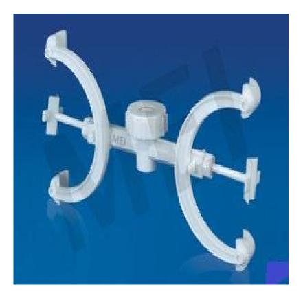
These Clamps are moulded in Polypropylene making it completely corrosion-proof. The spring loaded jack in the middle provides a vice like grip to the Burette and prevents it from slipping. Two tapered wedges are provided to ensure firm grip on roads having dia 1/2" or 3/8".
