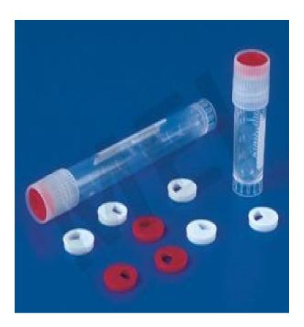
These Coders available in different colors can easily fit into the cap of cryo vials for color identification of different samples.
