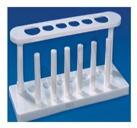
This autoclavable Stand is perhaps the most commonly used Test Tube Stand in various laboratories. For better visibility, this 6 places rack is end supported by 2 columns. The top plate has 2 holes for holding 25 mm dia test tubes, four holes to hold 16mm dia tubes where as the base has corresponding hemispherical wells. It also has six vertical pins for drying tubes. Another option available in this section is a test tube stand
