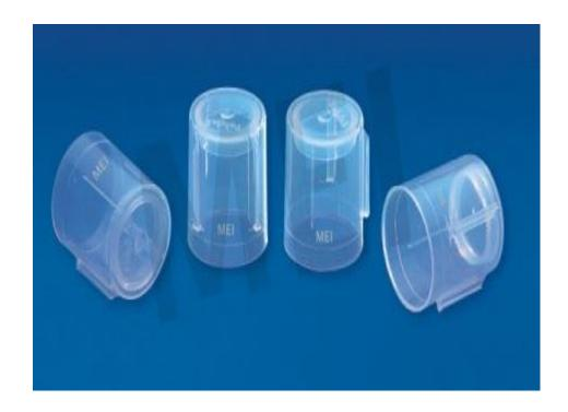
This transparent polypropylene cap for Test tubes proves to be an excellent protection to the contents to the tubes. The grooves inside the cap tighten the fitting on the tube while the outer grooves would hold identification labels. The built in seal ring would set in the tube making the combination a leak proof one.
