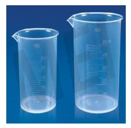
MEI Lab Beakers molded in polypropylene, have excellent clarity and very good chemical resistance. These autoclavable Beakers have prominently raised graduations on the outer surface. Pouring a solution becomes very convenient because of its tapered spout
