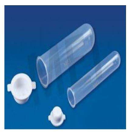
MEI Lab Centrifuge Tubes with rounded bottoms are moulded in polypropylene and Polycarbonate These tubes have excellent clarity and are strong enough to be used up to 50,000xG. These tubes can be autoclaved, however, repeated autoclaving in PC tubes reduces their mechanical.
