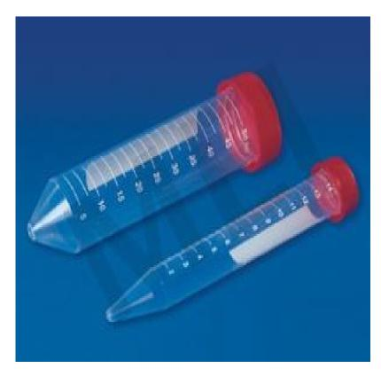
Centrifuge tubes with conical bottom are available in two sizes i.e. 15ml. & 50ml. Moulded in Polypropylene, these tubes are clear, strong & safe. These autoclavable tubes are provided with printed graduations on the outer surface. The built in seal ring in the cap makes these tubes absolutely leak proof. These tubes can withstand forces upto 7500Xg & 12000Xg for 15ml & 50ml. tubes respectively. These tubes are available sterilized as well as non-sterilized.
