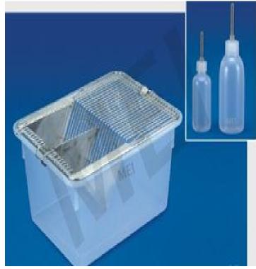
Avaiable in two different sizes, these Cages provide excellent shelter for different animal species in the laboratory. The metallic top provides proper ventilation and has provisions for feeding the species.
