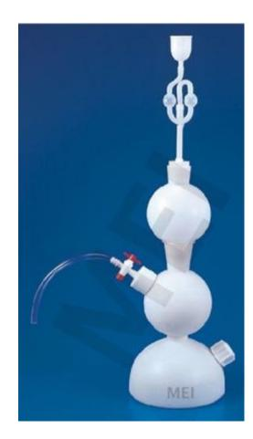
MEI Kipp's Apparatus made of Polyethylene has three main portions. The top portion is fitted with a thistle funnel and a bulb structure through which dilute acid can be poured which reacts with a metal sulphide In the base of the Apparatus. H2S gas then evolved collects in the middle dome from where it can be released through a leak proof stopcock fitted with a self lubricating PTFE plug. The base is provided with a residual outlet fitted with a cap for easy cleaning.
