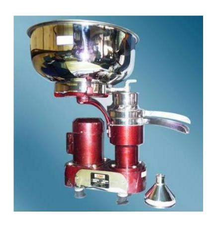
"MEI - 02" CREAM SEPARATORS HAND OPERATED, LISTER TYPE, AS - 9 MODEL SEPARATION CAPACITY 165 LITERS PER HOUR. SKIM MILK PAN, CREAM PAN AND FLOAT CHAMBERS ARE MADE OF MILD STEEL DULY TINNED. BOWL MADE OF SPECIAL STEEL AND FITTED SS DISC. TANK MADE OF ALUMINUM & HAVING APPROX 20 LITERS CAPACITY. 20-22 DISCS IN BOWL
