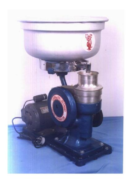
"MEI - 04" CREAM SEPARATORS LISTER TYPE HAND DRIVEN CAPACITY 60 LITERS PER HOUR. SKIM MILK PAN, CREAM PAN & FLOAT CHAMBERS ARE MADE OF MILD STEEL DULY TINNED. BOWL MADE OF MILD STEEL FITTED WITH S.S. DISC. TANK ALSO MADE OF MILD STEEL .HAVING CAPACITY 6-7 LITERS. 9-10 DISCS IN BOWL
