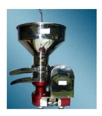
"MEI - 08" "MEI" CREAM SEPARATOR ELECTRICALLY OPERATED AS-107 MODEL. ALFA TYPE SEPARATION CAPCITY 300 LITERS. H. SKIM MILK PAN, CREAM PAN & FLOAT CHAMBER ARE MADE OF STAINLESS STEEL. BOWL MADE OF SPECIAL STEEL AND FITTED WITH MIRROR FINISH SS DISC. TANK MADE OF ALUMINIUM & HAVING 30 LITRE CAPACITY. ELECTRIC MOTOR AC 50 CYCLES, 220/230 VOLTS, SINGLE PHAS
