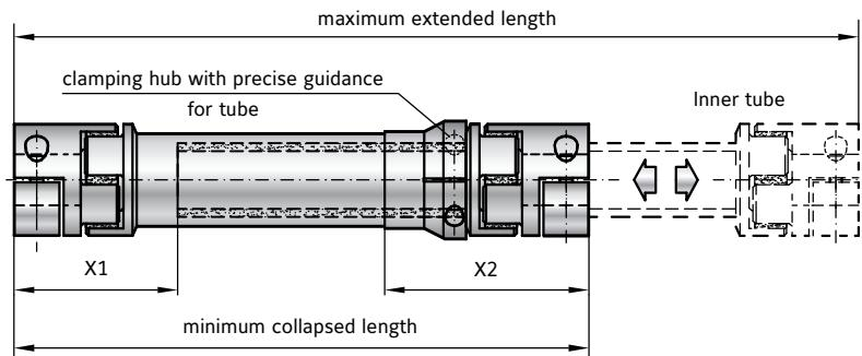
$$\text{Minimum collapsed length} = \frac{\text{maximum extended length} + \text{dimension } (X_1 + X_2)}{2}$$
