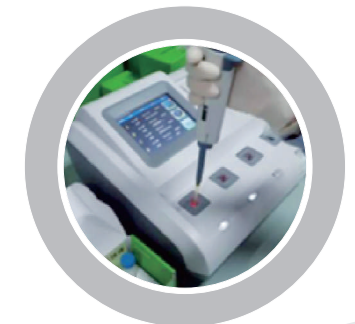
Step three Pipette anti-serum into the cuvette
