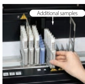
Set the rack containing additional samples and move the END rack to the right of the newly added rack.
