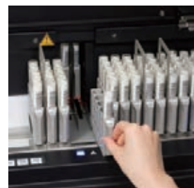
Set the tray on the rack sampler and start measurement.
