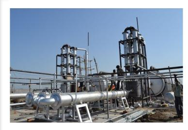
The pyrolysis plant is a machine converts mainly waste plastic/tyre to fuel oil. The raw material is waste plastic or waste tyre. The raw material will be heated in a reactor. When the oil gas goes into the condenser, the oil gas will be condensed into liquid oil/crude oil.
