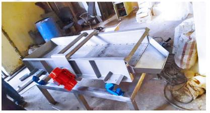
High-frequency vibrating screens are the most important screening machines primarily utilized in the mineral processing industry. They are used to separate feeds containing solid and crushed ores down to approximately 200  $\mu$ m in size, and are applicable to both perfectly wetted and dried feed.
