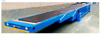
A Telescopic Conveyor is a perfect material handling equipment for an easy and efficient loading and unloading of goods such as cartons, packages, bags, crates, etc. Telescopic conveyor systems are also known as extendable conveyors due to their expandable booms designed to reach inside of vehicles in a safer and quicker way.
