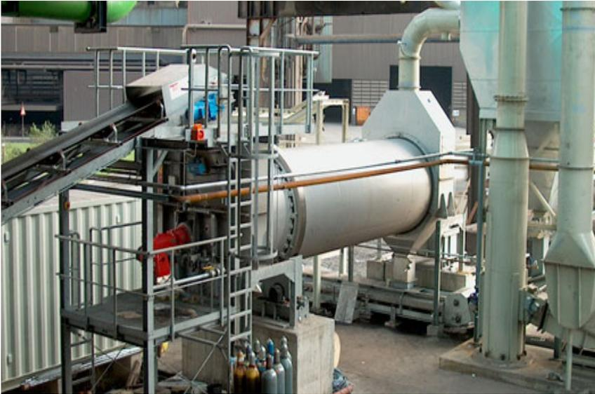
Rotary vacuum dryer is a horizontal cylindrical jacketed shell with hollow agitator, rotating in close clearance. A batch operation, drying is done under vacuum, heating is through jacket. The dryer offers a simple but effective method of drying wet cakes and sometimes slurries.
