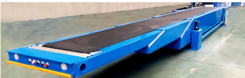
A Telescopic Conveyor is a perfect material handling equipment for an easy and efficient loading and unloading of goods such as cartons, packages, bags, crates, etc. Telescopic conveyor systems are also known as extendable conveyors due to their expandable booms designed to reach inside of vehicles in a safer and quicker way.
