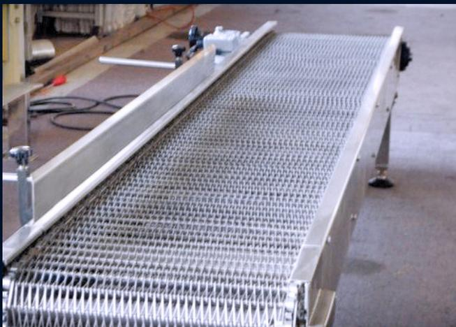
Wire mesh belt conveyors can be used in a variety of conditions to convey hot, cold, or oily products in oven, cooling, carrying cold items from a freezer, hot food items or other special conditions. A variety of belt types can be used depending on the application. It's designed to interface with existing conveyor systems and is custom engineered from standard components.
