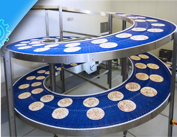
Spiral conveyors transfer loads from level to level quickly and efficiently, without interrupting the conveying process, without extra manual handling or transfers to other equipment. They're ideal for mezzanines, multilevel buildings, or elevated conveyor lines.
