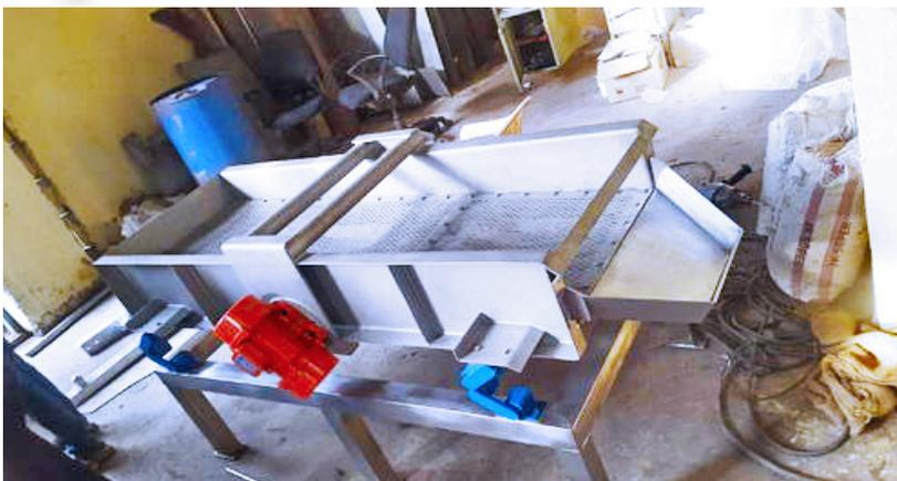
High-frequency vibrating screens are the most important screening machines primarily utilized in the mineral processing industry. They are used to separate feeds containing solid and crushed ores down to approximately 200  $\mu\text{m}$  in size, and are applicable to both perfectly wetted and dried feed.
