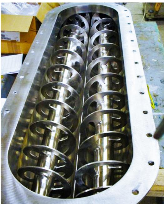
Multiple Diameter Screw Feeder / Conveyors consist of a screw feeder with an extension conveyor. ... When the bulk material reaches the extension conveyor the trough loading decreases and the bulk material is conveyed to the discharge.
