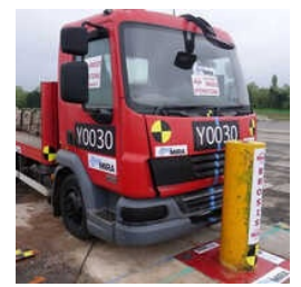
Force B12fb Crash Rated Fixed Bollards
