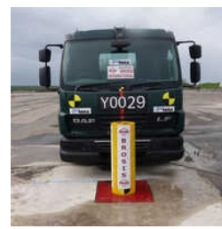
Force B8 K8 Crash Rated Bollards
