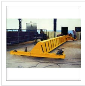
Overhead EOT Crane
