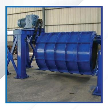
About Roller-Suspension Concrete Pipe Machine
