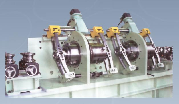
First ever, Rotary Sizing Mill (RSM) Supplied by KUSAKABE ELECTRIC & MACHINERY COMPANY LIMITED, JAPAN has been commissioned at APL Apollo Tubes Limited at their plant at Hosur, Tamilnadu. This equipment, first of its kind in India, is capable of achieving accuracy & precision as high as required for Dynamically balanced tubes & Surface finish as good as achieved by cold drawn process for most demanding customers.
