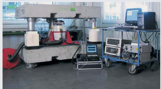
BILZ test bench (1600 Newton X-Y-Z Shaker)
