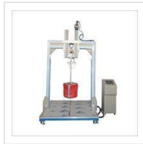
Chair Seat Drop Test Machine
