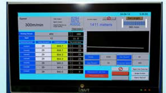
SCREEN Showing Uniform Tension from start to end of Beam
