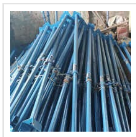
Scaffolding Adjustable Props
