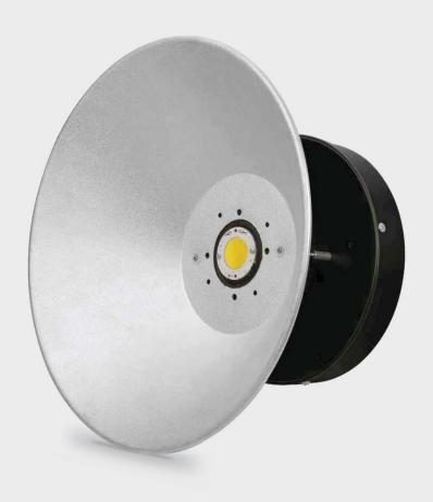
A high output led highbay fitting with active cooling & consistent color performance. Aluminum pressure die cast body & heat sink in durable corrosion resistance, anti-fading, anti-scratch electro static thermo painting finish with high purity metallized reflector for optimum light output.
