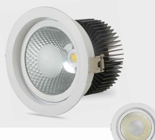
A high output led recessed downlite with active cooling & consistent color performance. Aluminum pressure die cast body & heat sink in durable corrosion resistance, anti-fading, anti-scratch electro static thermo painting finish with high purity metallized reflector for optimum light output.
