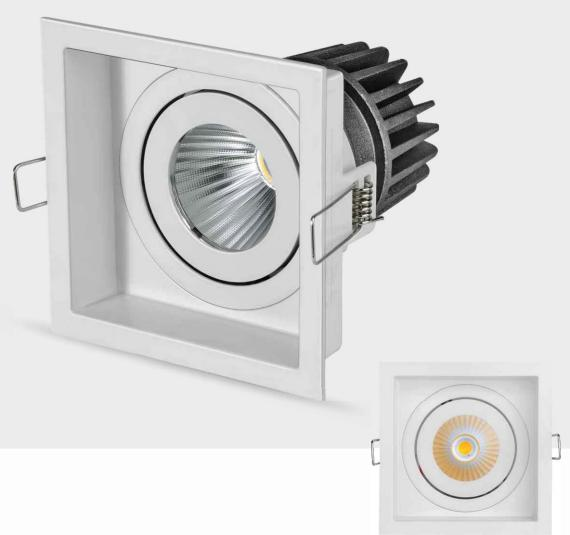
A high output led recessed downlite with passive cooling & consistent color performance. Aluminum pressure die cast body & heat sink in durable corrosion resistance, anti-fading, anti-scratch electro static thermo painting finish with high purity metallized reflector for optimum light output.
