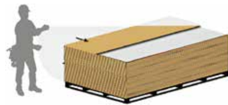
Panels must never be stacked in partial sizes in widths also. All Panels should be stacked of the same length sizes.
