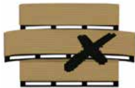
Panels must never be stored in an uneven lengths.
