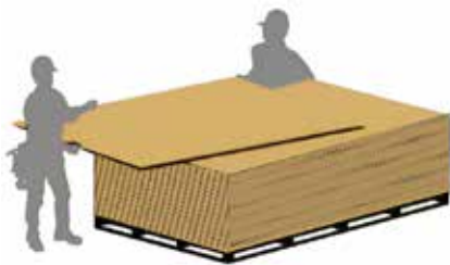
Panels must never be slided over while storing to avoid scratching.
