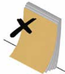
Panels must never be stored inclined by the wall side.
