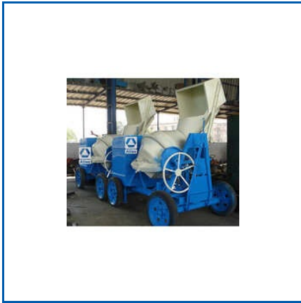
MANUAL CONCRETE BATCHING PLANT
