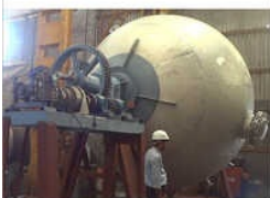
Rotary Spherical Digester
