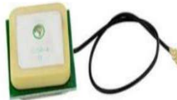
GPS Internal Antenna (25mm* 25mm)
