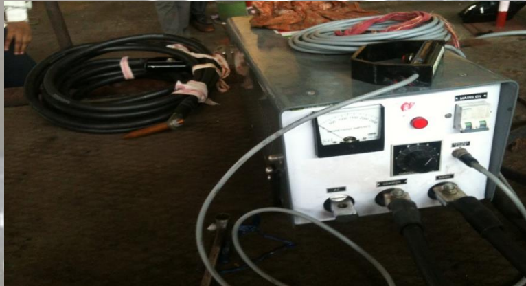
ITE's MPT equipment for Coil/Prod method
