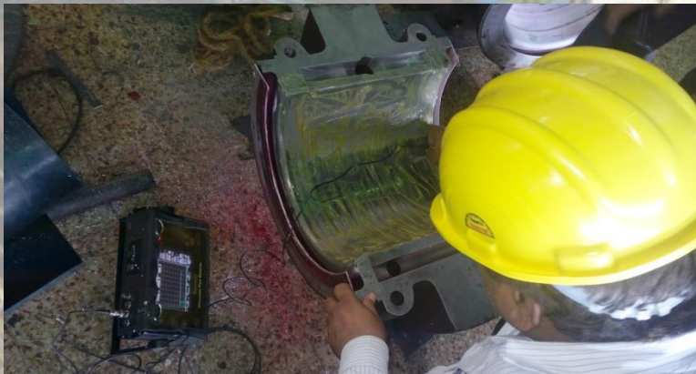
Ultrasonic Testing of Bearing being carried out
