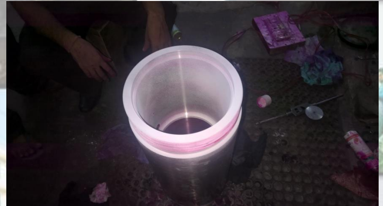
Visible Dye Penetrant Testing of Forged/Machined item
