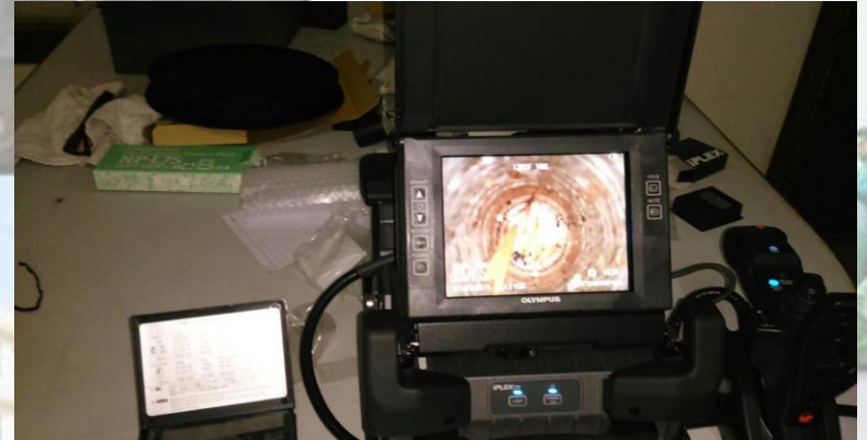
ITE's Industrial Borescope with 18 meter length and 6 mm dia.
