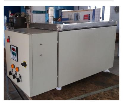
Steam Humidifiers are custom designed and tailor made in complete S.S.304 parts with heavy duty, high density electrical immersion heaters with complete automation controls to generate semi saturated steam at atmospheric pressure, of various capacities.
