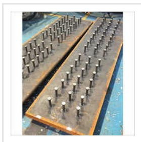
Anchor Plates Shear Connector Stud
