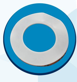
Polytetrafluoroethylene (PTFE). It is composed of elastic materials such as compressed asbestos sheet, rubber, etc. and PTFE envelope cover. These are successfully used in chemical plants, glass/glass lines equipment due to their high temperature, corrosion resistance. These are used in areas where an envelope of pure PTFE is required to protect the exposed joint edge from corrosive attack or for applications where hygiene conditions are essential.
