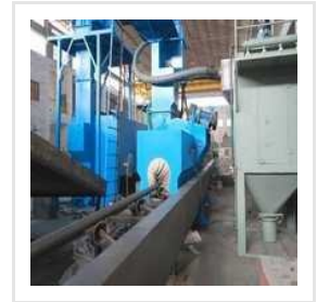
Rod Bar Shot Blasting
