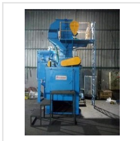
Tumbblast Shot Blasting
