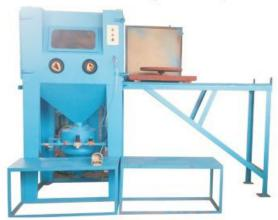
PB is recommended for fast cleaning, for removal of heavy rust and corrsion using coarse abrasive, it is most suitable for etching the surface needed for rubber-lining, FRP lining and metal spaying. Castings and forgings are cleaned speedily. Blast pressure can be controlled from 30 to 90 psig. Almost all types of coarse and medium size abrasive can be used depending upon application.
