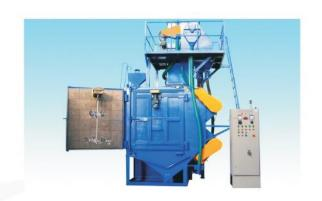
The Dust particles generated in the system are collected in a number of Plated Bags in a dust collector. Clean air is exhausted through an exhaust fan. The Plated Bags are cleaned by Pulse type Reverse Jet air cleaner controlled through Solenoid Value and the collected dust particles fall in a dust bin and taken out for disposal from time to time.
