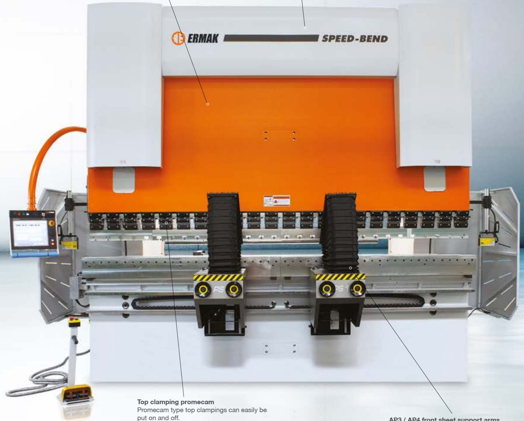
AP3 / AP4 front sheet support arms CNC controlled support arms reduces your bending time significantly and is a great help for perfect bending.
