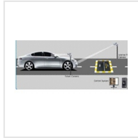
UNDER VEHICLE SCANNING SYSTEM (UVSS)
